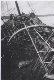
The foredeck of the Berwick Castle, viewed from amidships, showing the collapsed saloon house, Captain's cabin and bridge in foreground
